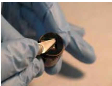
Figure 7-6. Removing the Spacer
