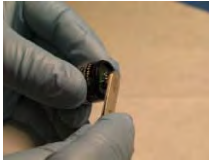
Figure 7–11. Pressing Down the PID Lamp
