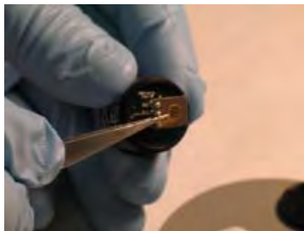
Figure 7-7. Removing the Cell Assembly
