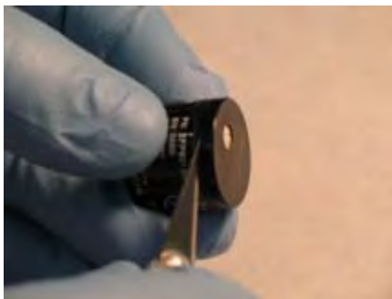
Figure 7-4. Removing the Filter Cap
