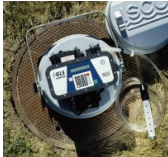
Shown here on a 23-inch manhole cover, the GLS Sampler is a compact 16.5 inches in diameter.
