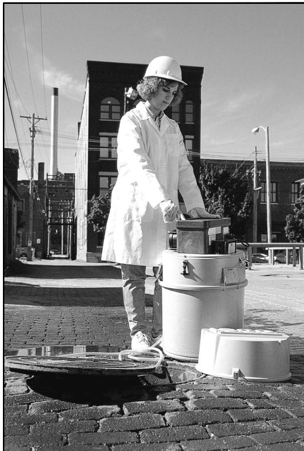
Figure 2-3 Placement of the Sampler Adjacent to Manhole
